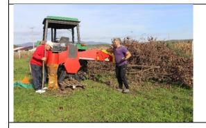
The chipper, which is connected to the tractor, is being used to cut branches up to 10cm into sacks which can be burned in house heating systems for Danny and Adopt-a-Friend families.
